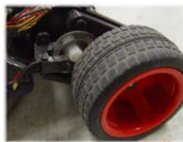
Optical encoder mounted to the motor output shaft
