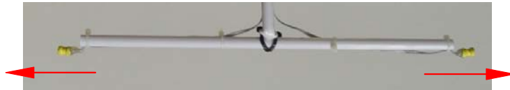
Map 4-9 An electromagnetic coil mounted horizontally
