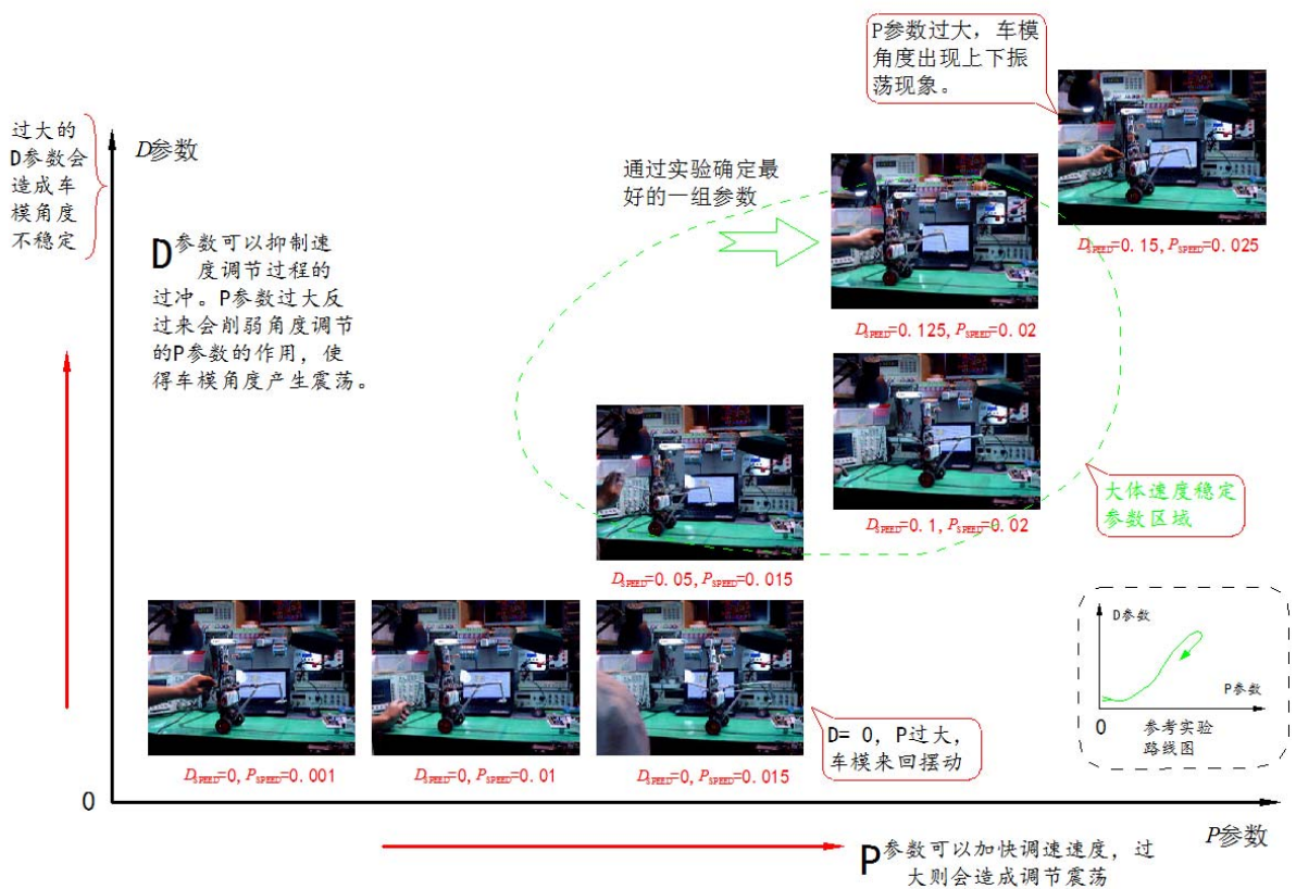
Map 6-22 Speed parameter adjustment process
