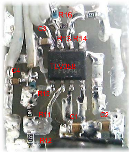
Map 3-15 based on LMV358 FIG detector circuit amplifying two physical channels
