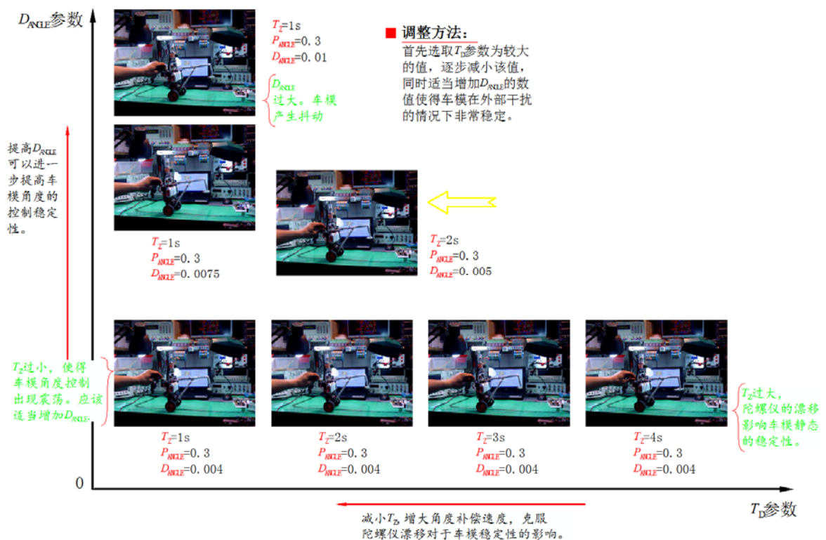
Map 6-24 Angle compensation time constant adjusting
